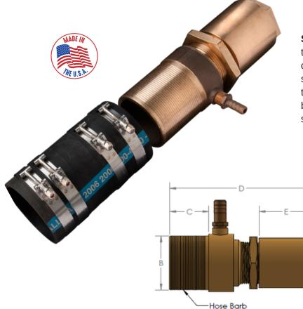
**SA Series** - Water fed self-aligning shaft seal that is safer and performs better than socalled "*dripless*" or "*packless*" mechanical seals. Compatible with most shaft tube (stern tube) arrangements. Refer to sizing guide below to determine correct part # based on shaft diameter and shaft tube size.
