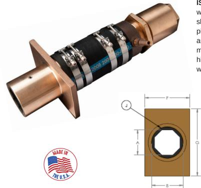
**ISB-SA Combo Series** - The perfect upgrade for boats with traditional bronze stuffing boxes. Our self-aligning shaft seal is attached to an intermediate shaft bearing (in place of existing stuffing box) offering improved safety and reliability over "*dripless*" or "*packless*" style mechanical seals. Proven performance for today's higher horsepower commercial and recreational boats with less noise and vibration.
