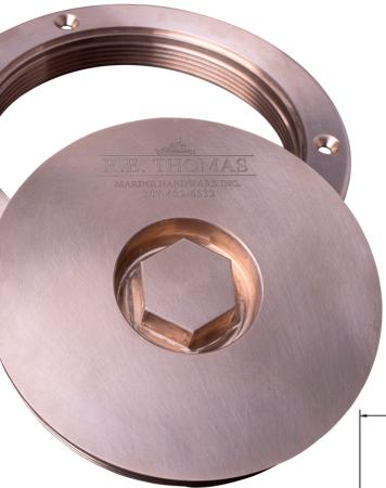
Bronze Deck Plates - Our heavy duty bronze deck plates feature a rugged ACME dual thread pattern to prevent stripping and cross-threading (similar to a firefighting hose connection). They also feature a rubber o-ring gasket to help ensure watertight integrity and are easily opened/closed with the included 1 1/2" socket.
